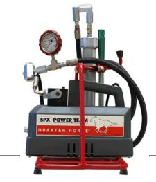
The Val-Tex 1400 is a rugged, light weight unit that is self priming and can be used in any position. The hydraulic system is equipped with an internal hydraulic relief and comes complete with sealant hose including 15,000 PSI, 2.5" 316 SS gauge and giant buttonhead coupler.
